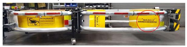
The STMS should always do an equipment check before leaving the yard. This includes all electronic displays and TMAs. Even slight damage can considerably degrade the performance of the TMA.
