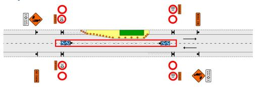
Centreline cones are used to stop road users crossing the centreline or where lanes have been shifted, form a new centreline to keep opposing traffic separated.
