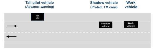
Shadow vehicles are required for the protection of TM crew and must be used whenever risk assessment identifies a shadow vehicle is required.
