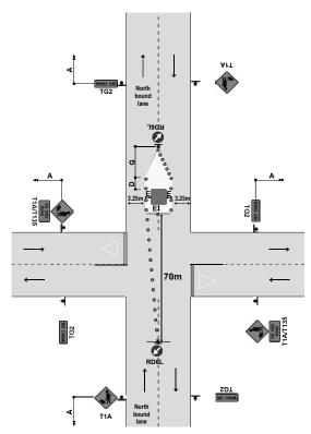
$\label{eq:decomposition} \mbox{Diagram showing the solution - 70m taper substituted by a 10m taper with positive traffic management$
